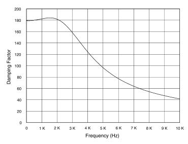
Figure 7.5 CTs 8200 Typical Damping Factor vs. Frequency
